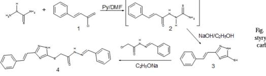
Fig. 1. Synthesis route of 1H-3styryl-5-benzylidenehydrazinocarbonyl-methylsulfanil-1,2,4triazole (Tz3a.7)
